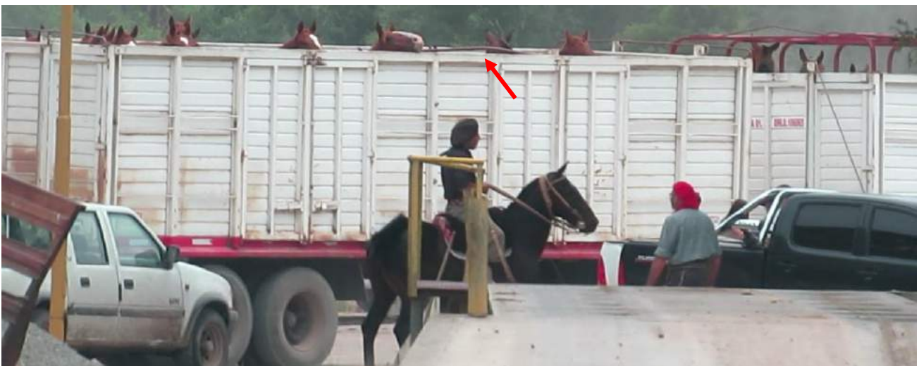
Very low metal bars in the trailer – risk of serious head injuries
